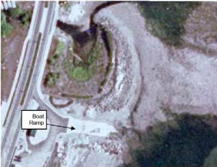
Figure B-1. Aerial view of Ken Forde Boat Launch showing rock groyne to the south and rock structure to the north (2007 orthophoto).
