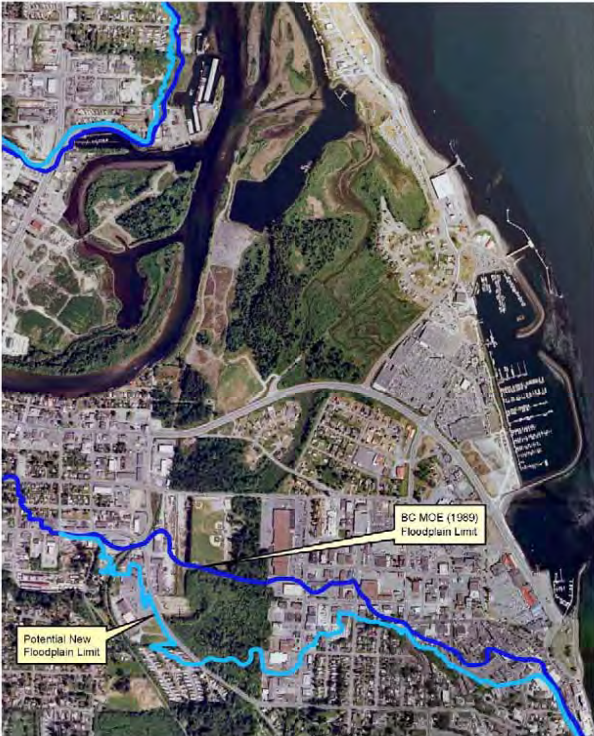
Figure 5. Floodplain extents based on existing mapping (Campbell and Quinsam Rivers, BC MOE, 1989) and on projected future sea level rise scenario.
