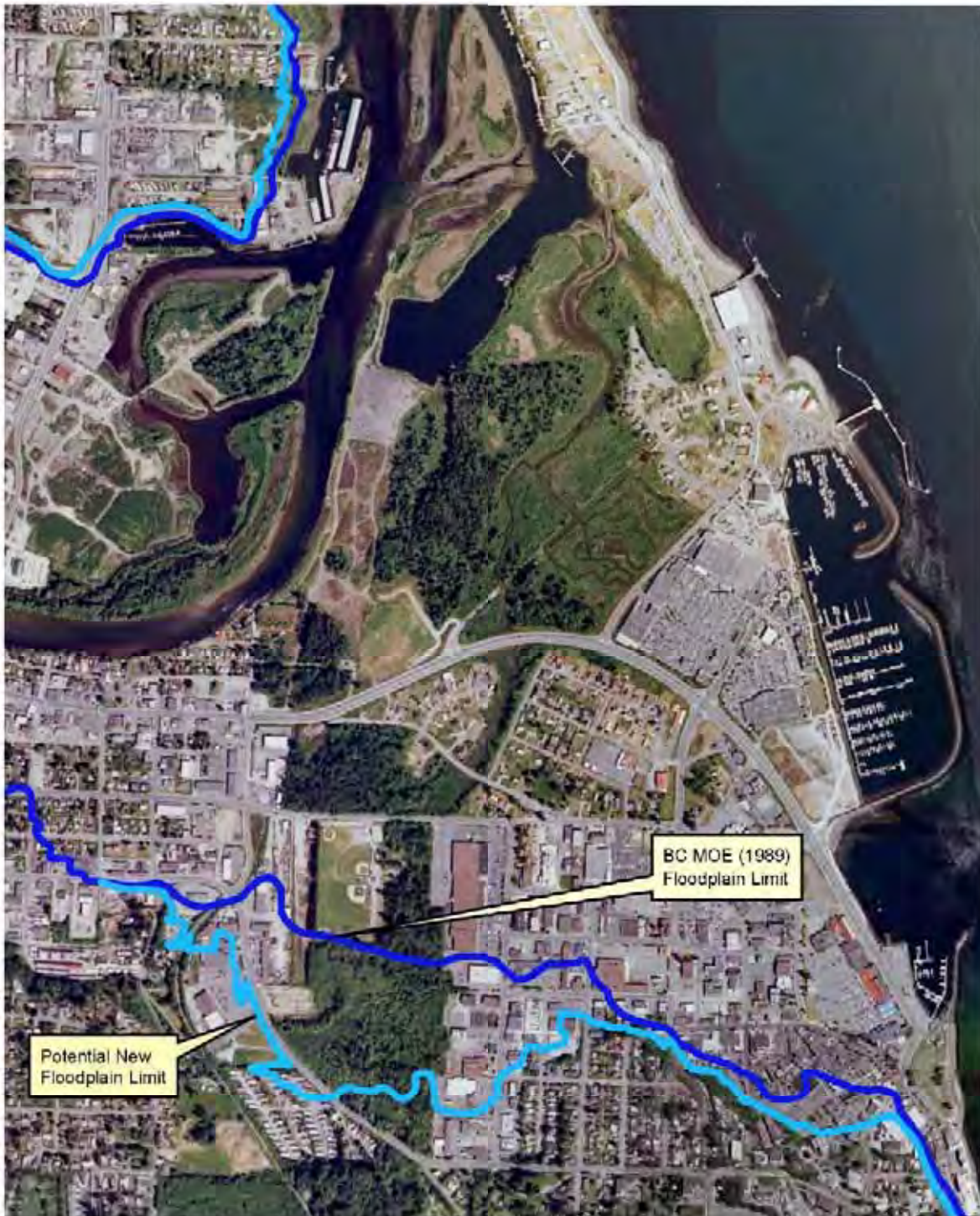
Figure A-25. Floodplain extents based on existing mapping (Campbell and Quinsam Rivers, BC MOE, 1989) and on future sea level rise scenario.
